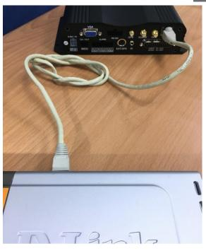
Connect with switch via RJ45 cable.
